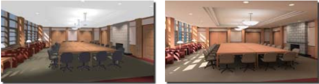
Figure 1. The image on the left was modeled and rendered by an architecture firm using 3D Studio. The image on the right is the same model rendered in Lightscape. Note the gradual gradation in the brightness of the ceiling from the window to the walls and how the ceiling picks up some of the color from the table and floor (color bleeding). Also note the soft shadowing around the table and ceiling coffers. While it certainly would be possible to obtain a similar quality image with 3D Studio as with Lightscape, it would require that the user have a good understanding of what the lighting should look like and then a good technical understanding of the lighting tricks and techniques required in 3D Studio to render them. With Lightscape's robust lighting interface and global illumination rendering, the process of lighting a scene and obtaining these effects is more intuitive. Designers simply set up lights the way they would want them in a real environment. The lighting effects are calculated automatically by Lightscape to produce a superior quality image that is closer to what this conference room would actually look like if built (Images courtesy of Zeidler Roberts Partnership, Toronto, Canada)
